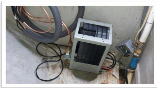
The first step per the instructions is to find a large deep cabinet with unused space in the back. I have a 32' C&C racer / cruiser. The cruiser part of the boat has a great layout with teak walls and teak & holly floor. The racer part of the boat means cabinets are a waste of space and don't exist let alone be large and deep. I opted to locate the 14" x 8" x 6" compressor in the large step in lasserette near the bulkhead adjacent to the ice box. The
